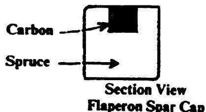
The ribs are mounted 45° to the flaperon spar to achieve torsional stiffness. The structure will be covered with light weight Dacron at 45°.
