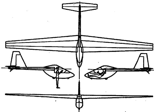
The goal in designing and building the Carbon Dragon was to try and bring foot-launch glider performance up into the lower range of sailplane performance.
