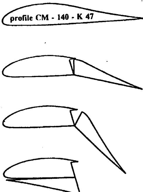
Moreover, he moved the axis of rotation to the lowest point. With this trick it is possible to tilt the flaps over 180° which reduces the package measurements for easier transportation ( see below).
