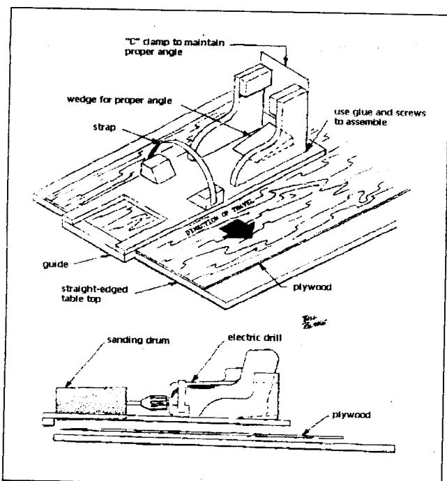
Here is a little gadget I came up with while searching for an easy way to scarf plywood for my project. It's simple, inexpensive and, above all, foolproof! All the other methods I have seen involve feeding the plywood into a saw or some other piece of equipment. This way, the plywood remains stationary.
