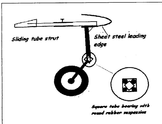
Laurie doesn't use fiberglass. His wheels feature a sheet steel leading edge section and a bracket, which holds the wing at the trailing edge. The design I have drawn shows the IS28 wheel, which fits on the wing tip end plate.
