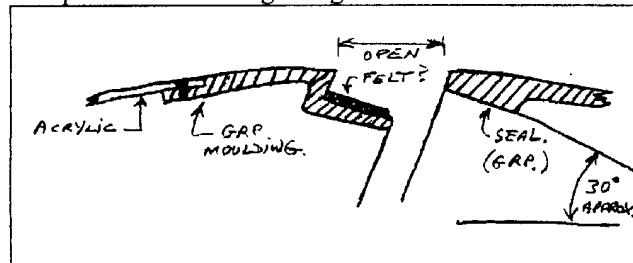
The ring type seals, at nose and rear, should seat on a cone of felt or similar material, set at about 30 degrees to the axis
