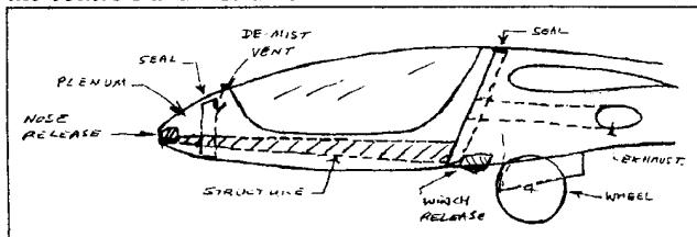
In the air it is also practical, although the rear seal and leakage needs to be improved. Unfortunately the MOBA-2 design, of a three-piece wing, makes this difficult to improve.
