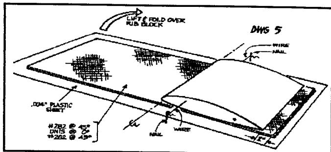
Note: We clamp the T.E. section of the wet lamination to the table so we can pull as hard as possible around the L.E., making sure that there are no wrinkles on the unis over the entire lamination.
