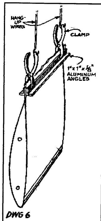
After proper cure, remove the clamps, aluminum angles and Mylar. Do not remove peel ply!
