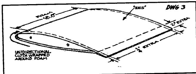
Now let's suppose that the cloth wrap measures 18.50" in width and 53.00" in length. We will need two of them (at  $+45^\circ$ ) and also the unidirectional cloth, called unis. In our case, the required thickness for the unis came to .080". Size them at 18.50" x 53.00".
