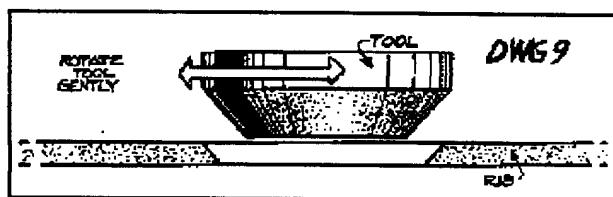
Any piece of softwood will do. Machine the conical area, dunk the conical surface in epoxy, shake excess and sprinkle with sand. After it has hardened, you'll have a very handy, 30° sanding tool. Holding the sanding cone with your fingertips, rotate the tool into rib holes with very light, even pressure...just enough to produce a 30° sloped edge. See Dwg 9.
