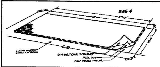
Cover with enough unidirectional (unis) cloth to get the required .080", making sure that the fibers are straight and run in the chord direction (0°). Do not disturb the bi-directional cloth below! We will refer to this unidirectional layer as 1 ply.
