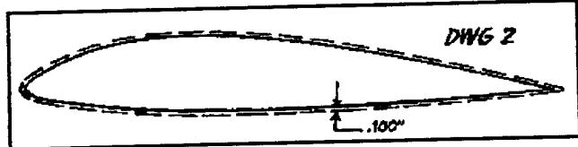
In our particular case, we do not have to consider just the thickness of the cap but also the thickness of the leading edge "D" tube, a.k.a. "Taco Shell." Let's suppose that we need two plies of #7781 glass, or better yet two of #282 graphite. At .010" each ply, we need to reduce the patterns by another .020" all around.
