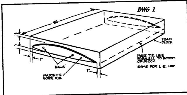
Remember that the foam block is going to be covered with unidirectional fibers (graphite or glass). For a 2 ft. chord, to be used on a small sailplane or light airplane, .080" is more than sufficient. That means that we must cut the foam blank .080" under size. All the popular CAD systems will automatically deduct the "cap" thickness at your command.
