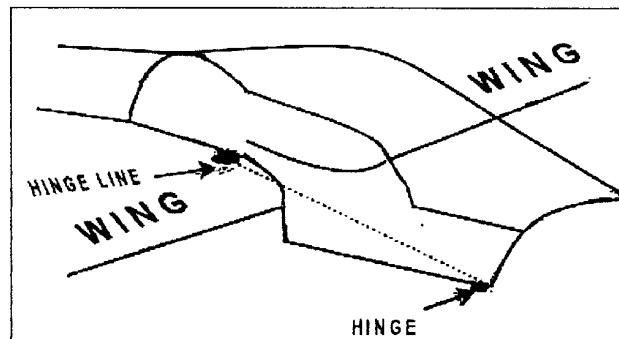
The canopy can be hinged if the hinge line is through the front corner and the top of the wing with the hinge line off set say 20mm out from the face of the canopy. This allows the section of the canopy that wraps around the front edge of the wing to lift away and rotate as the canopy is opened.
