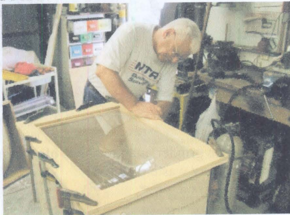
A panel of cast acrylic is clamped between the upper and lower frames. >>
