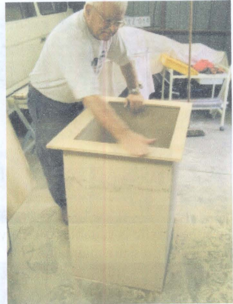
Fitting the inner supporting frame to the top of the box.
