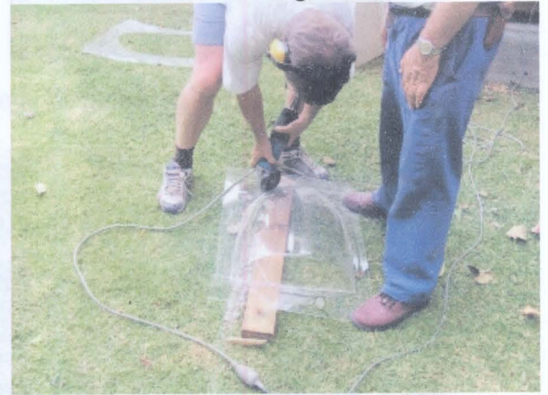
An angle grinder and metal cut-off disc are used to cut away waste material
