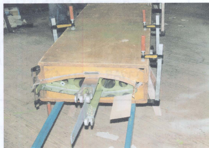
Wing all clamped up. Note wooden stick at leading edge. The sheet of balsa wood adjusts a defect in the jig.
