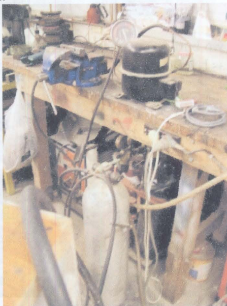
Vacuum rig consists of an old fridge compressor, a scuba tank for storage and an automotive vacuum guage, Mole grips clamp the delivery line.
