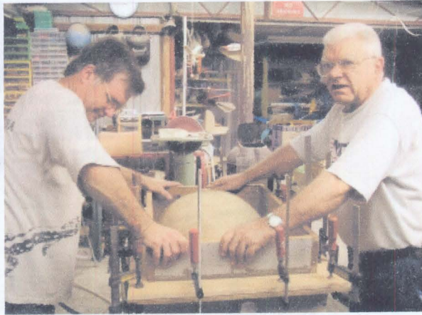
Once the acrylic is suitably soft the vacuum is applied and pressure maintained.>>
