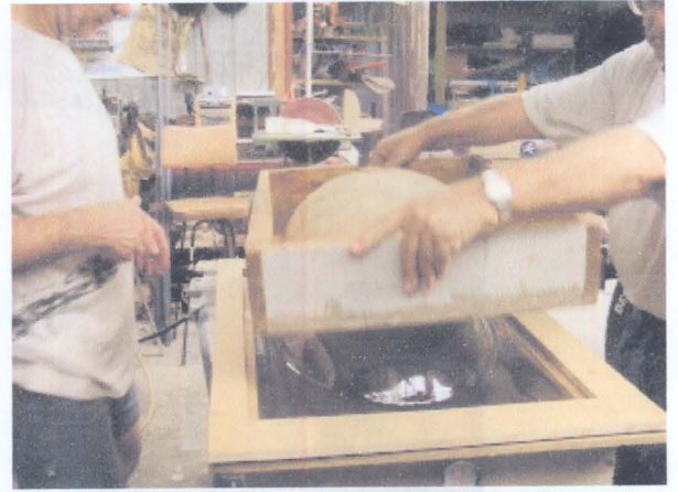
After removing the heat the acrylic is allowed to cool a little before releasing the vacuum.
